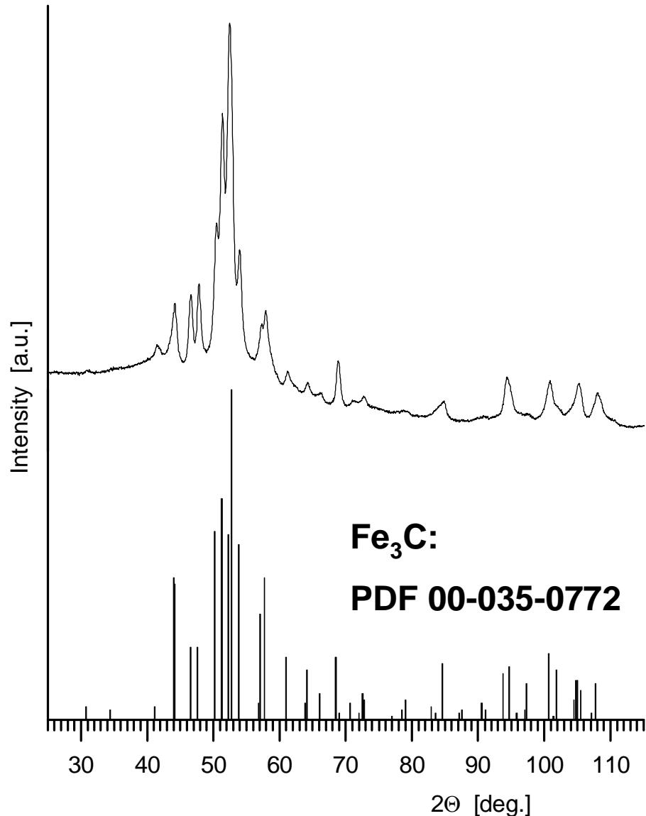
$\text{Fe}_3\text{C}$  clearly detected:
