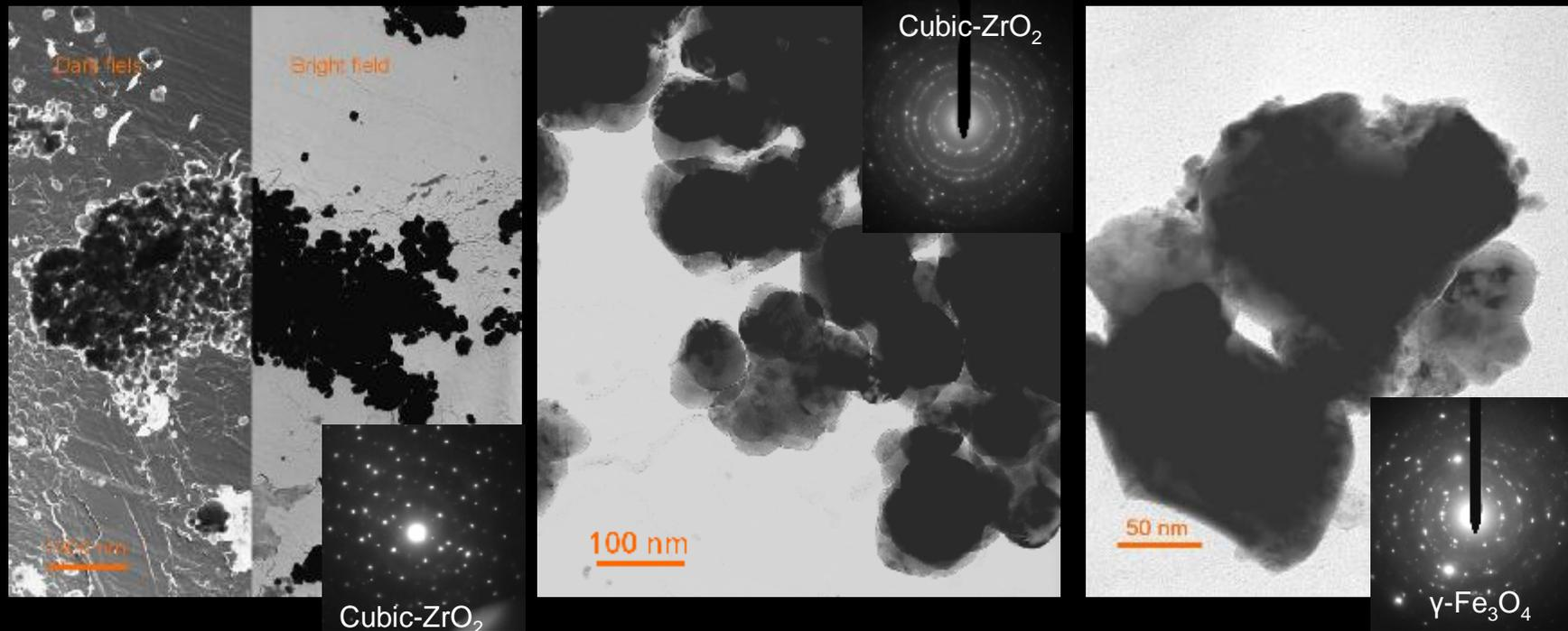
Selected area diffraction pattern from fine particles was identified as cubic form of ZrO<sub>2</sub>. The clusters of Fe<sub>3</sub>O<sub>4</sub> are disseminated in zirconia matrix.
